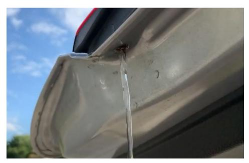
78. Once water infiltrated the Taillight Assembly and causes damage to the lighting components contained therein, the only way to fix those components is to replace the entire
