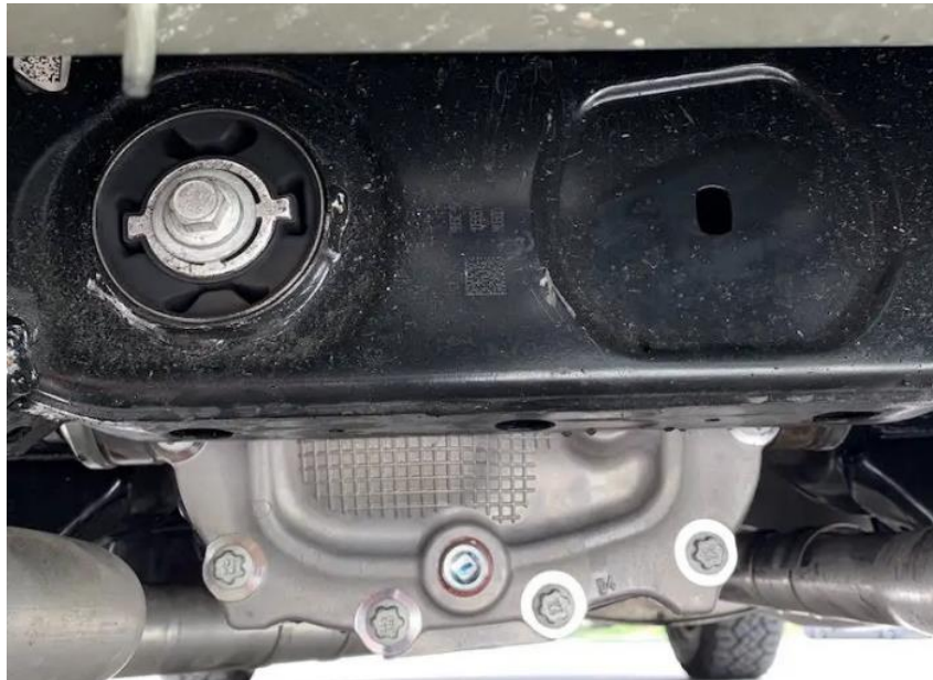
1 Fig. 2 – Close Up of One Rear Axle Mounting Bolt in Fig. 1, as Attached to Vehicle
