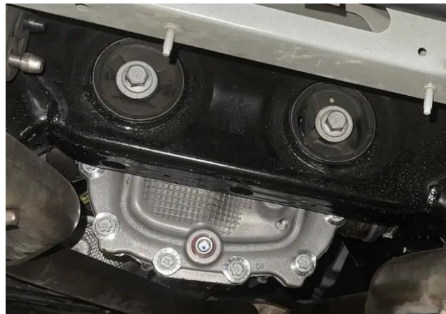
13 Fig. 4 – Close Up of Two Rear Axle Mounting Bolts in Fig. 2, as Attached to Vehicle 14
