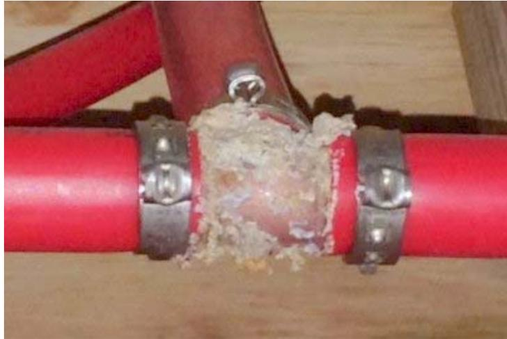
36. The below photograph is a side view of a NIBCO ASTM-F1807 PEX Fitting from Monica's home which demonstrates the corrosion and scale affecting the NIBCO brass fittings.
