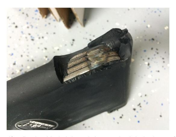
18. Even the weights that had not yet broken appeared cracked and on the verge of breaking.
