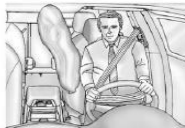
If the vehicle has a front center airbag, it is in the inboard side of the driver seatback.
