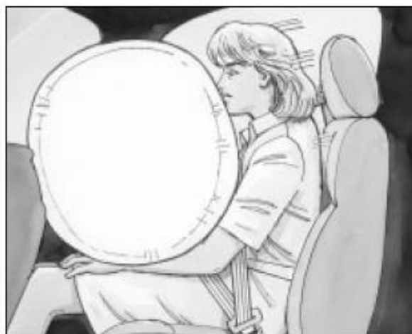
The right front passenger's frontal air bag is in the instrument panel on the passenger's side.
