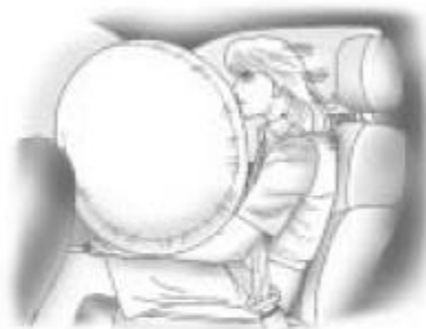
The right front passenger frontal airbag is in the instrument panel on the passenger side.
