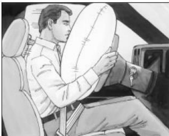
The driver's frontal air bag is in the middle of the steering wheel.
