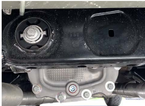
Fig. 4 – Close Up of One Rear Axle Mounting Bolt in Fig. 3, as Attached to Vehicle
