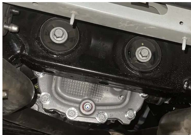
19 20 21 22 23 24 25 26 27 28 Fig. 2 – Close Up of Two Rear Axle Mounting Bolts in Fig. 1, as
