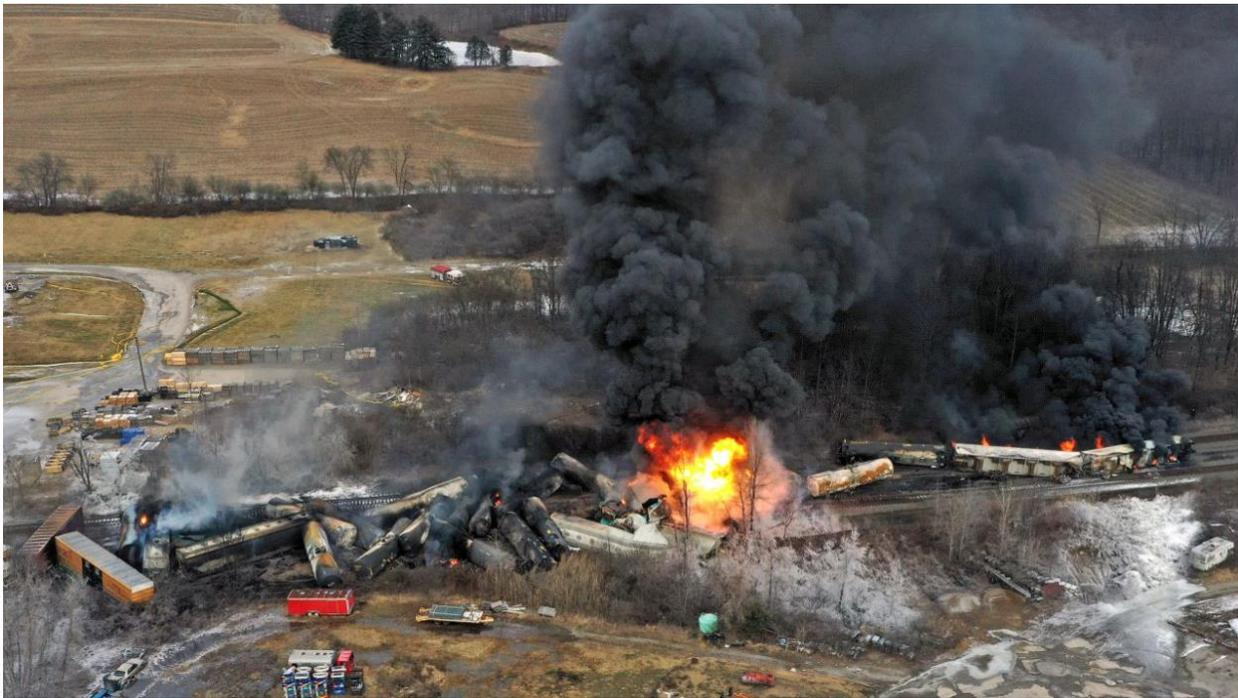
6. The heat from the blaze increased pressure in the Vinyl Chloride cars, leading to an activation of emergency relief valves design to vent vinyl chloride to the atmosphere to relieve pressure under emergency conditions.
