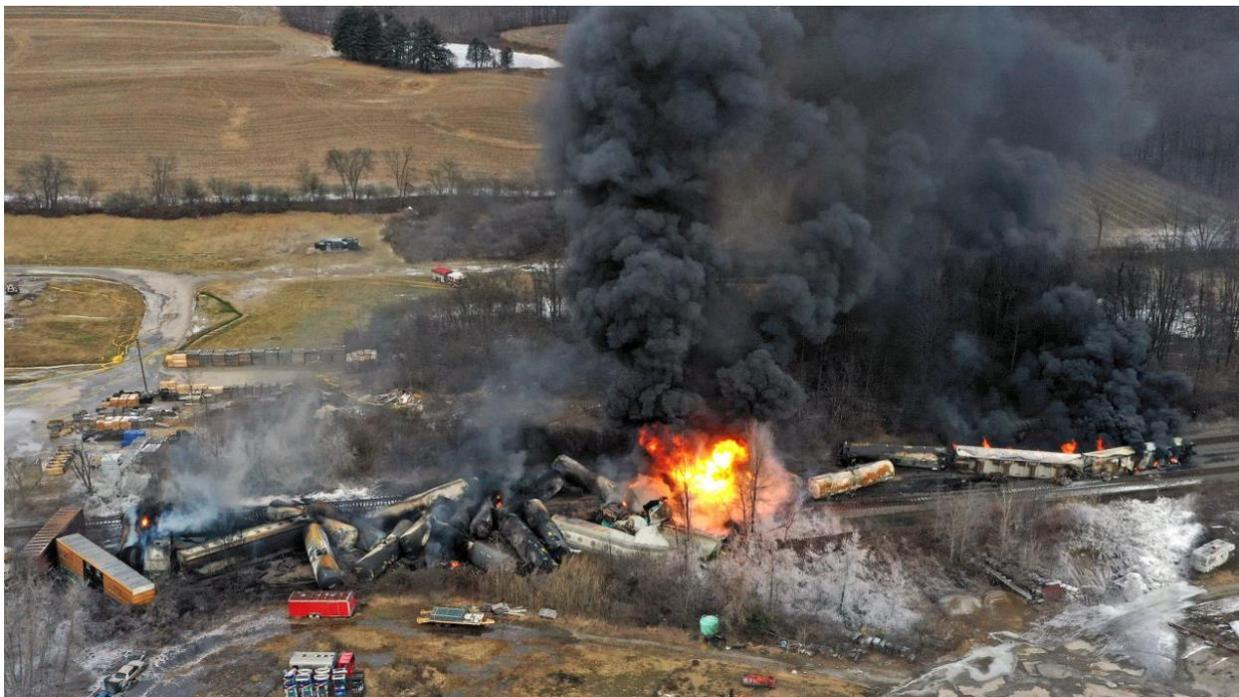
6. The heat from the blaze increased pressure in the Vinyl Chloride cars, leading to an activation of emergency relief valves design to vent vinyl chloride to the atmosphere to relieve pressure under emergency conditions.
