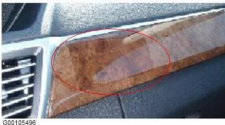
Fig. 1: Example Of A Faded Area Behind Removed SRS Label
