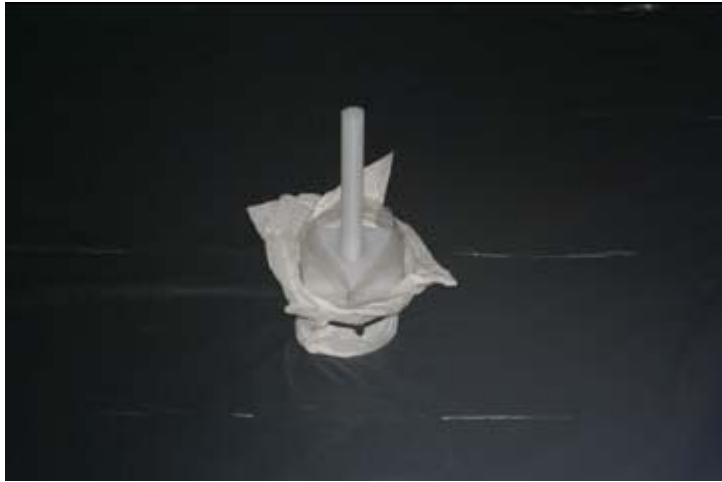
Figure 3: Weight with 1-quart polyethylene storage bag, a wipe (this is a paper towel for demonstration purposes only), and a cable tie
