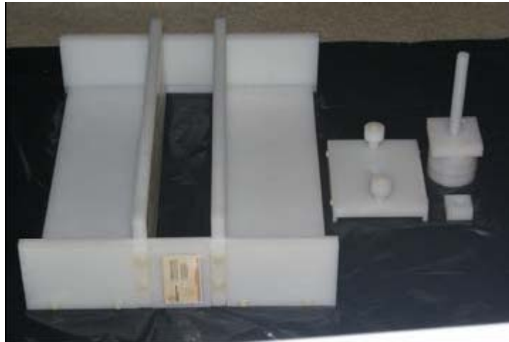
Figure 2: Sampling device frame, slide, weight and nut
