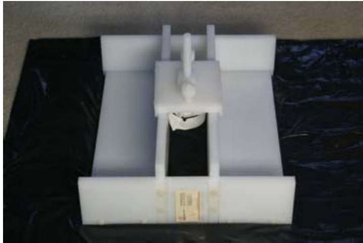
Figure 5: Slide placed on device frame rails.
