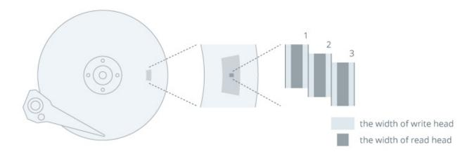
11. CMR HDDs "delivery excellent random-access performance," and are as such "widely used not only in PCs but also for online storage applications." CMR is used in most standard HDDs.<sup>5</sup>
