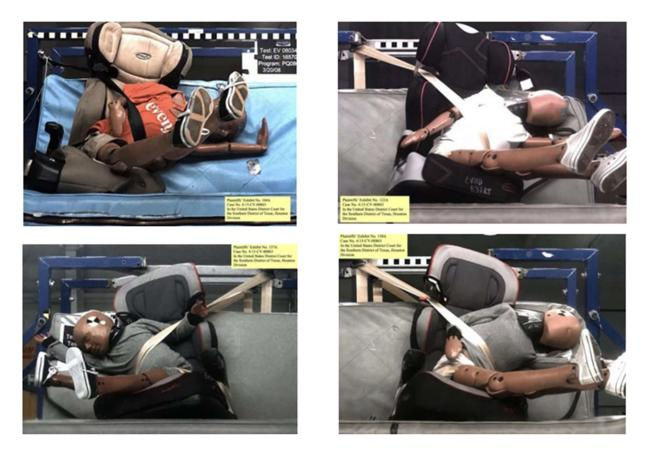
51. These images show the seat belt slipping off the dummy's shoulders and instead tightening around its abdomen and ribs. This kind of violent movement at high speed can cause serious damage to a child's internal organs, head, neck and spine, including paralysis or death.
