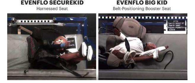
32. In the test of the SecureKid, the dummy's head and torso remained entirely within the seat's confines. By contrast, in the test of the Big Kid, the seat belt slipped off the dummy's shoulder, and the dummy's head and torso flailed far outside the seat.
