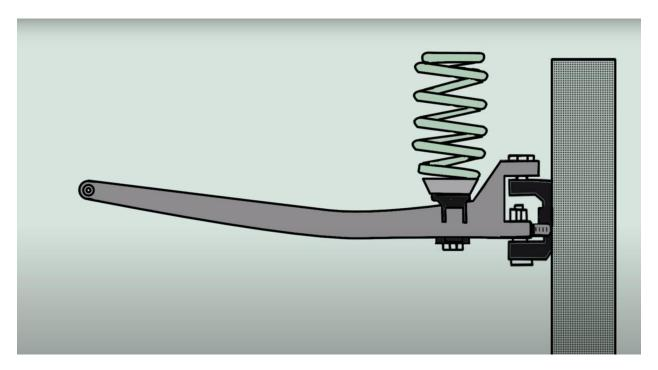
36. The next diagram shows weight applied to the I-beam suspension and the resulting negative camber of 2 degrees.
