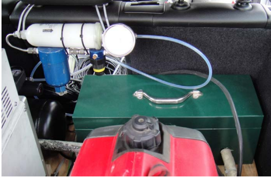
Figure 3.30: PPS setup, the sensor is housed within the green box, top left : pressurized, dried and HEPA filtered air supply for PPS
