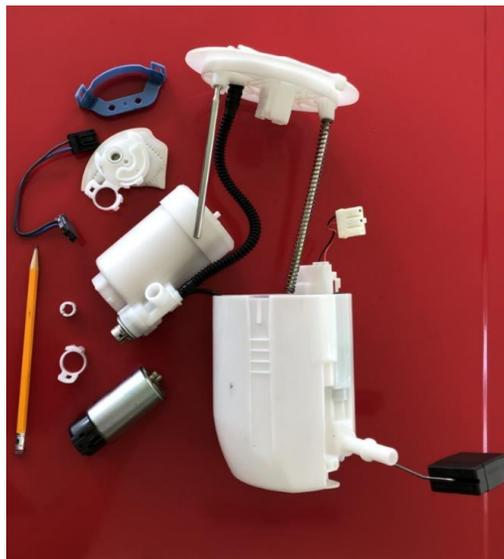
163. The fuel pump module's housing protects the fragile internal components that fit together like puzzle pieces within the module.
