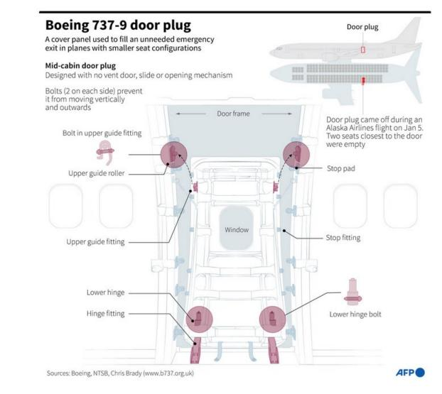
2.6 <u>Missing and/or defective bolts</u>. On information and belief formed after reasonable inquiry, and subject to further investigation and discovery, The Boeing Company delivered the subject 737-MAX 9 to Alaska Airlines, Inc. without properly securing the plug to the airframe, and/or one or more of the bolts and/or seals required by design to secure the door was or were
