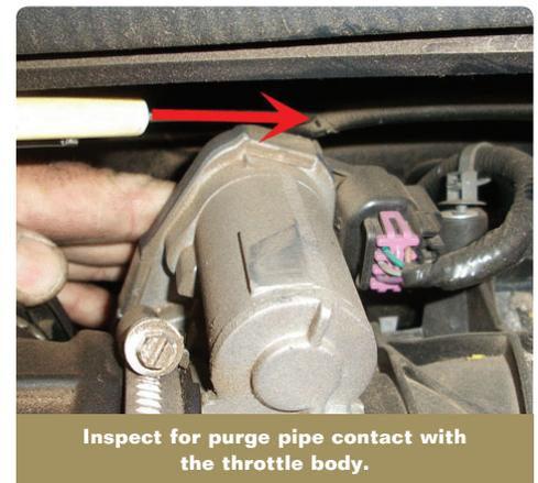
Inspect for purge pipe contact with the throttle body.
