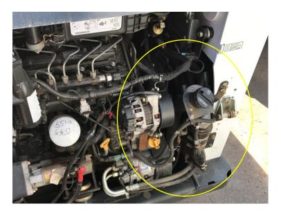
5. Compounding the problem is the heavy-duty and rugged work for which Loaders are intended to be used. Common Loader uses include pushing and lifting ground or gravel and navigating over ditches and rugged, uneven terrain. Such operations create more opportunities for the drive belts and the hydraulic fluid and fuel lines to make contact, increasing wear and on the
