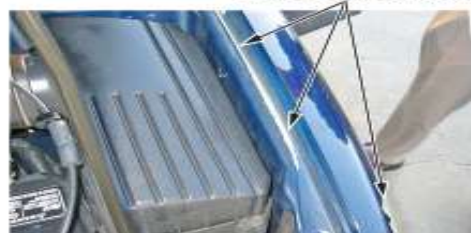
14 Example of paint peeling off the top of the left fender.
