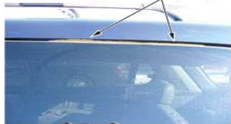
12 Example of paint flaking off the upper half of the left quarter glass.
