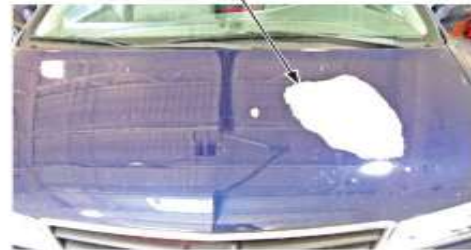
10 Example of paint peeling off the hood.
