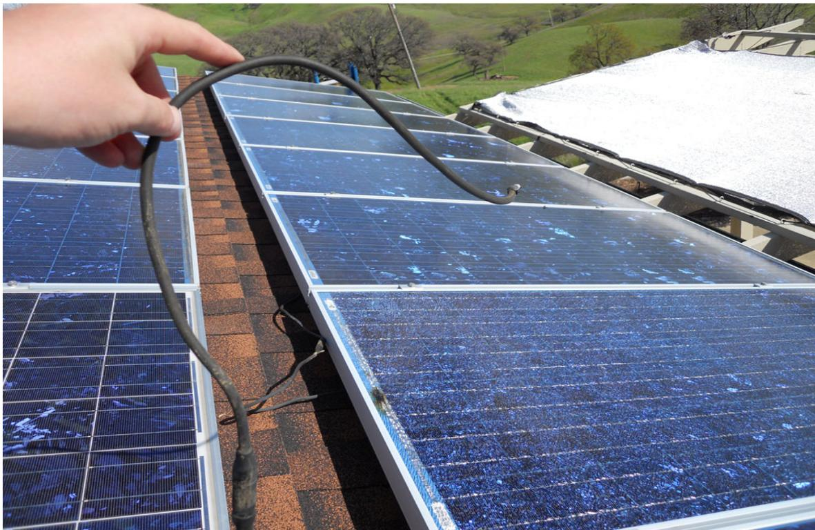
**Model No. BP SX3 150S – Burned Connecting Cable Associated with Junction Box Failure**
