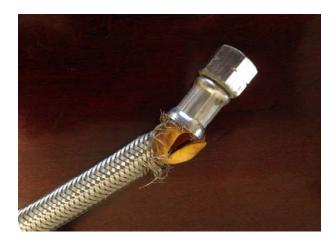
61. Chloride stress corrosion is a well-known and generally accepted phenomenon in the scientific community and in the plumbing industry. Fluidmaster knew or was reckless in not knowing that by selecting an inferior grade of stainless steel, combined with low-pressure inner rubber tubing, it was creating a product designed to fail. These defects were present at the time of manufacture and sale to Plaintiffs and the Class who had no knowledge of the defects.
